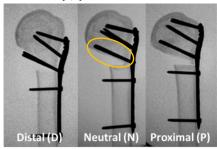
**Fig 1:** Fluoroscopic images of the 3 groups tested in the experiment. The screws circled in yellow are inserted into the calcar.
