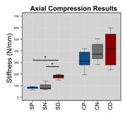
**Fig 3:** Plots of stiffnesses for Sawbones and cadaveric specimens during the 0° axial test. Significant differences between groups are marked with a \*.
