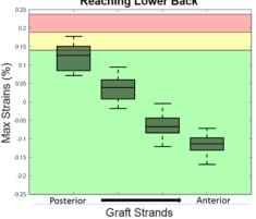
**Fig 3:** A box and whisker plot showing the distribution of maximum strains from simulations of reaching the lower back. The most posterior graft strand is strained the most and may break because it overlaps with the experimentally determined failure zone (yellow and red), as determined with in vitro testing.
